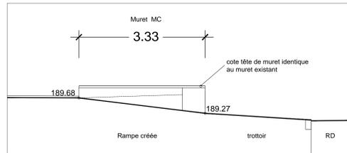
ELEVATION SUR MURET MC - Face Rampe - 1 / 50 e
